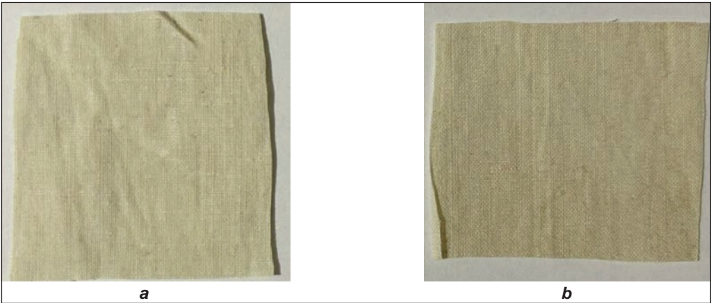
Fig. 1. Image of the heritage sample: a – before; b – after treating it with the AgNPs dispersion
